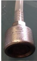
If the filter is dirty, this sucking side hose strainer also need to be cleaned after operation.
