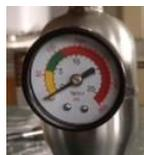
Pressure meter is seen during the operation. Standard operational pressure is 5kg/cm<sup>2</sup>
