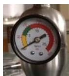
When turn on the motor, pressure level should be around 5kg/cm<sup>2</sup>
